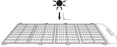
Position the solar panel in most direct angle towards the sun as possible.
